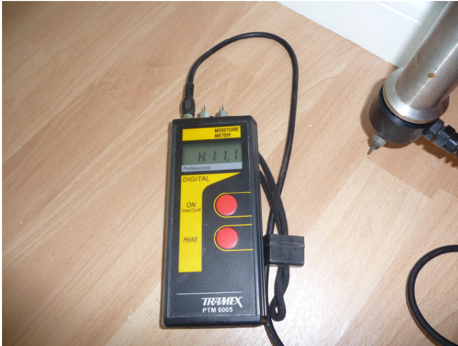
20. Measuring screed at 11.1% WME at far end of lounge
